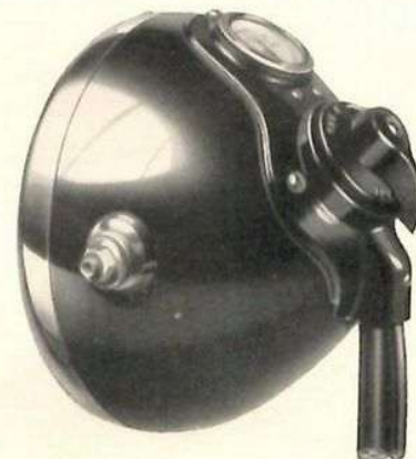
LUCAS No. DU42M PROJECTOR SUPPLIED WITH SWITCH, ILLUMINATED AMMETER, DIP-BEAM DEVICE, AND WITH GIRDER BRACKETS AS ILLUSTRATED ON H52 LAMP ON OPPOSITE PAGE.
