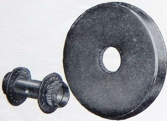
Brake drum and hub showing method of attachment
