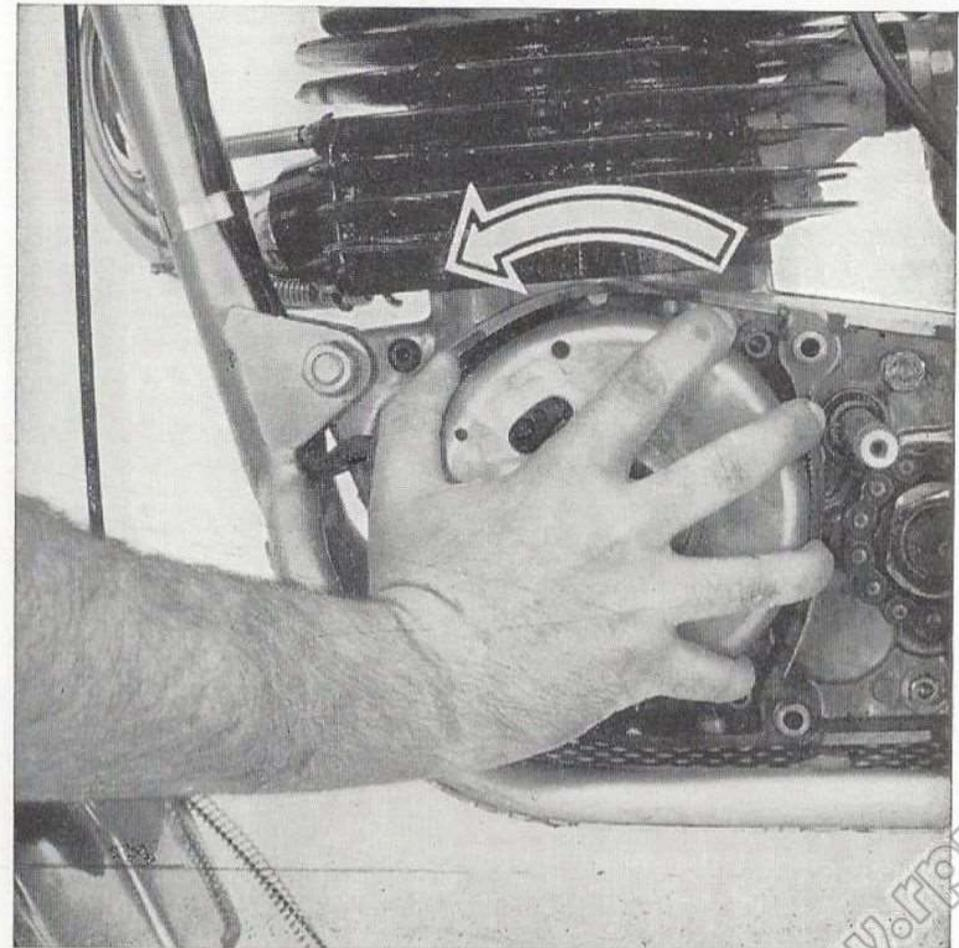
Loosen the clamp positioning the electrical wires beneath the magneto flywheel. Pull back the plastic insulator to expose the connection between the red wire and the black wire.
